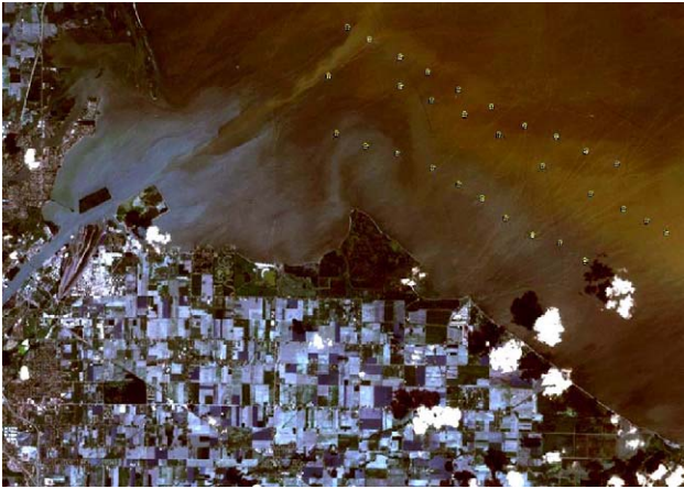
Fig. 1. LANDSAT 7 ETM+ image (bands 1, 2, and 3 displayed as blue, green, and red, respectively) of part of the July 1, 2000, Path 20 Row 31 frame, showing collection sites of 30 water samples as black buttons with yellow dots in Maumee Bay, OH. North is toward the top.
